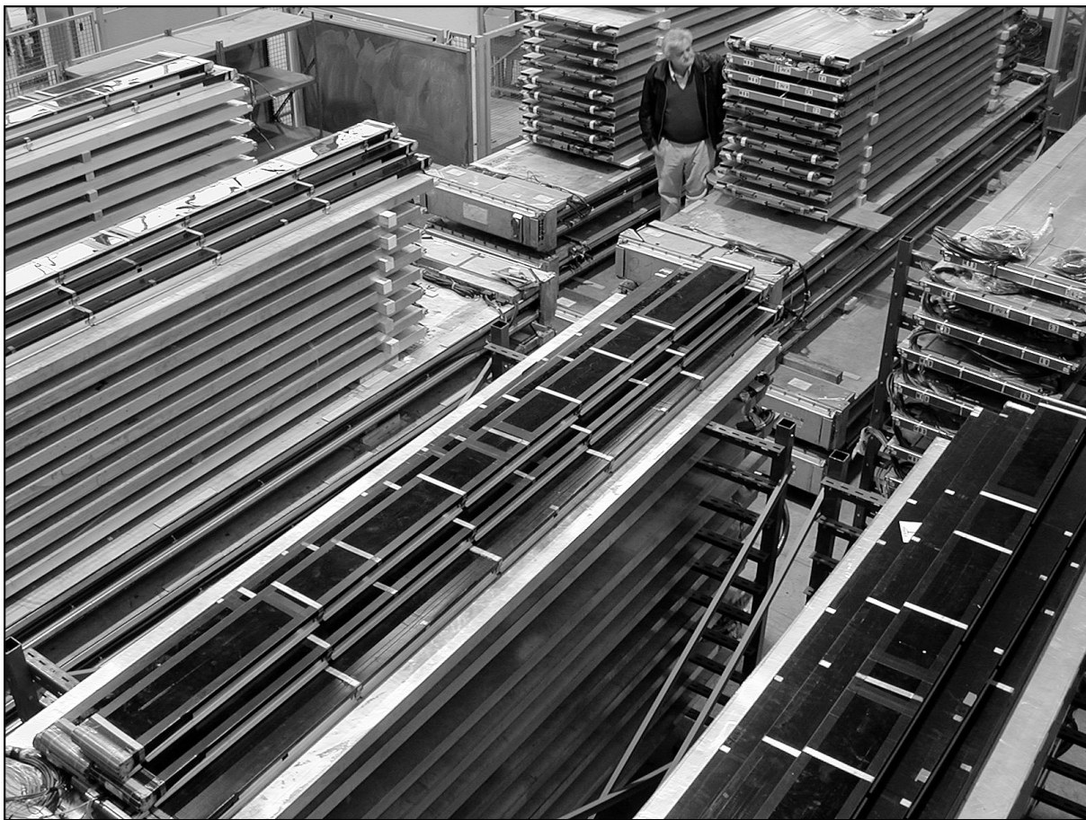
Figure 4.1. UA1 and DELPHI muon chambers in hall 167.
