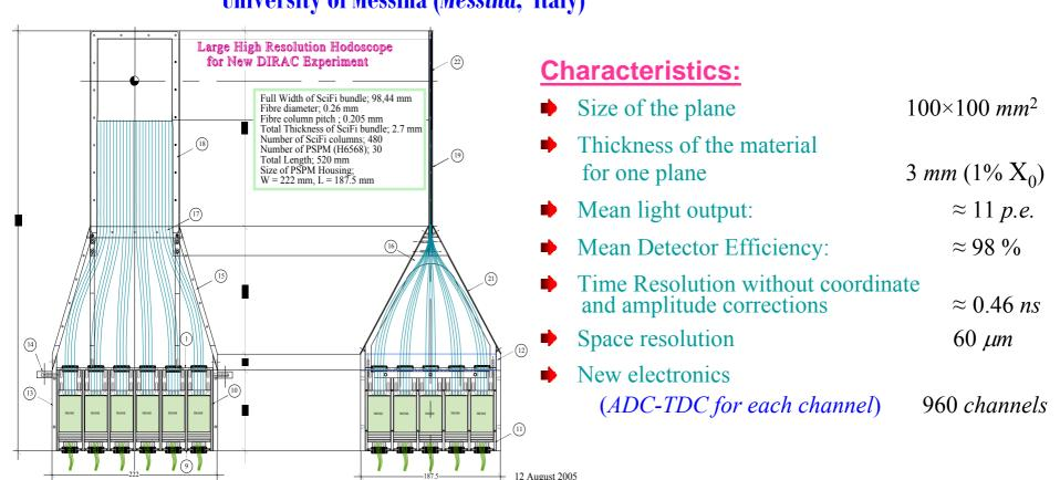
Two new SFD detectors were tuned on the test beam T11 during August-September 2006, installed at the DIRAC setup and checked.
