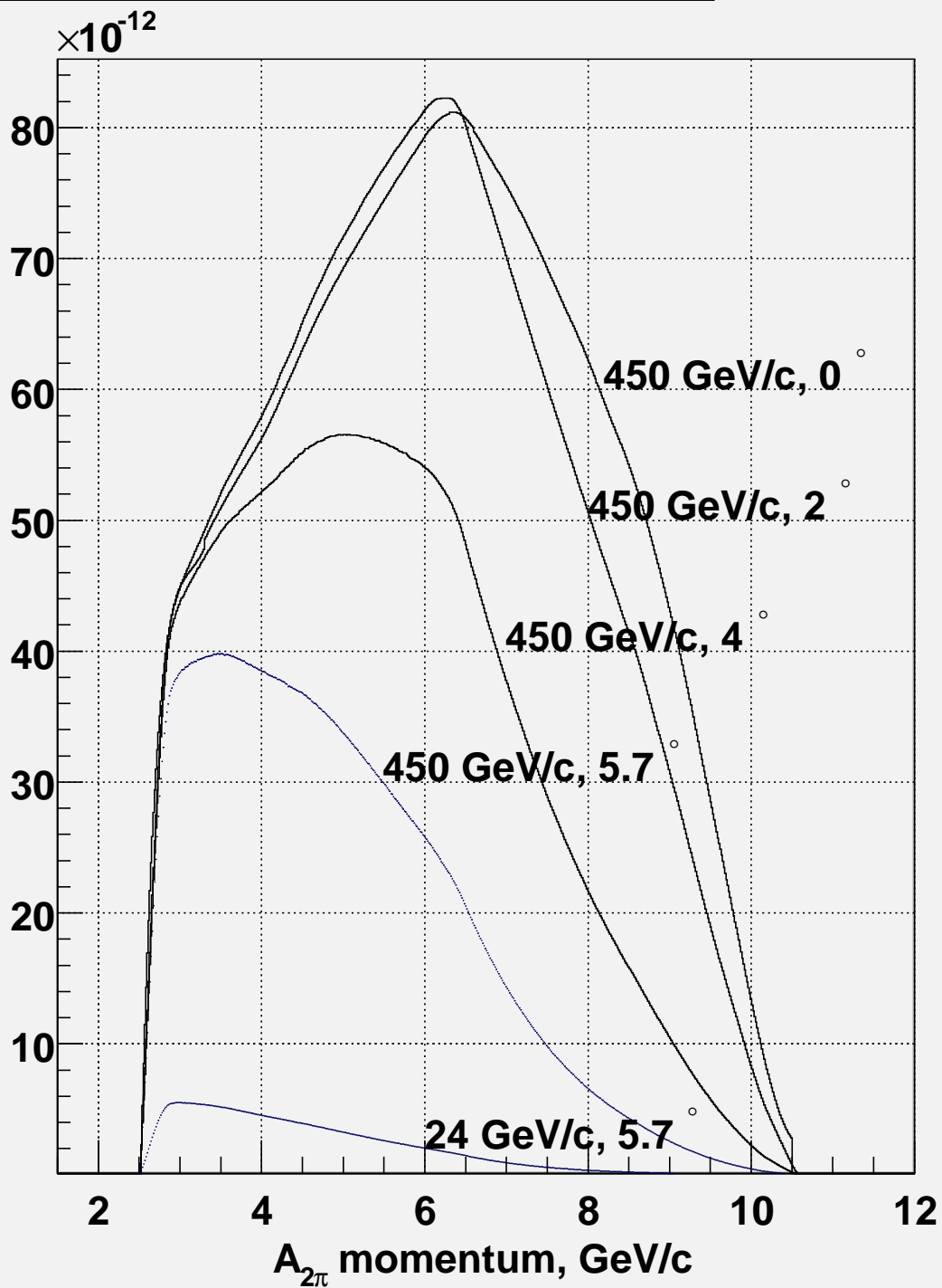
Figure 14: Yields of A_{2\pi} atoms per one p-Ni interaction with taking into account their acceptance value and calculated correlation factor R at the proton momentum 450 GeV/c and emission angles \theta_{lab} = 0^\circ, 2^\circ, 4^\circ, 5.7^\circ and at the proton momentum 24 GeV/c and emission angle \theta_{lab} = 5.7^\circ as a function of the A_{2\pi} momentum.
