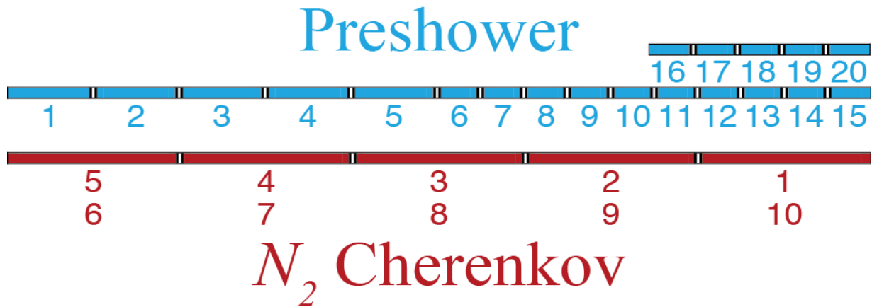
Figure 3. Relative positions of the N_2 Cherenkov and Preshower elements. The numbers show the PMT positions (left arm)
