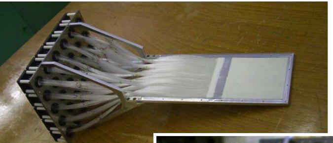
Sensitive area 98.5 x 107 mm<sup>2</sup> consists of 480 columns of 8 Scintillating Fiber of 0.26 mm in diameter
