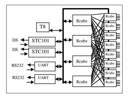
Fig 7. 32 way switch block diagram
