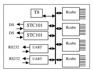
Fig 9. Four 8 way switch block diagram
