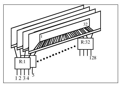
Fig 4. 128 Node switch based on 32 valent modules
