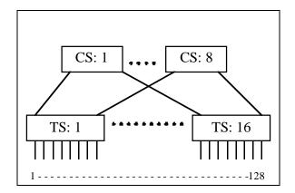
Fig 3. 128 Node switch based on 16 valent module
