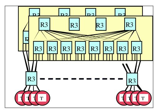
Fig. 13. 64 Node testbed structure
