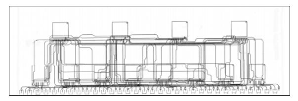
Fig 6. HS link PCB interconnections
