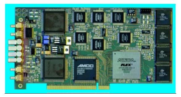
Fig. 12. Photograph of the PCI HS-link Interface
