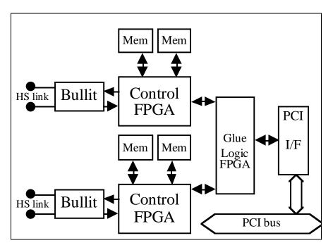
Fig 11. Block Diagram of the PCI HS-link Interface
