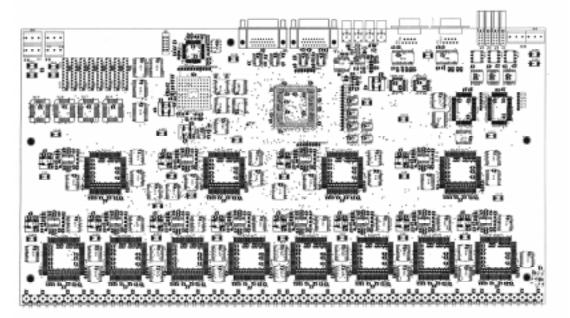
Fig 8. 32 way switch printed circuit layout
