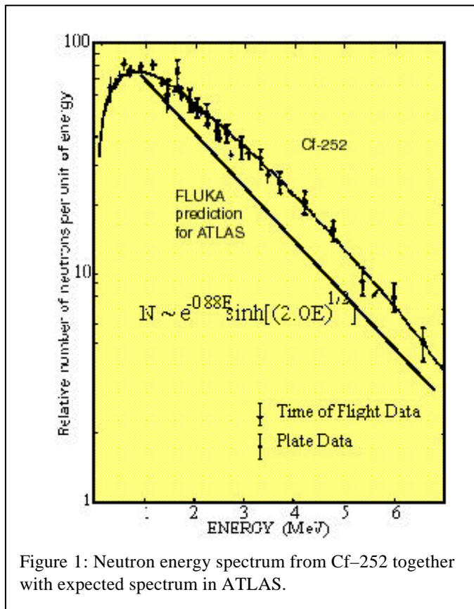
Figure 1: Neutron energy spectrum from Cf-252 together with expected spectrum in ATLAS.
