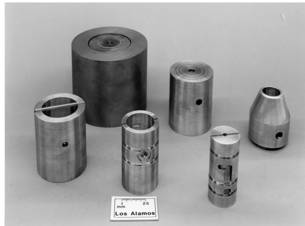
Figure 6. Concentric copper cylinders with coolant passages, brazed using low-thermal-expansion sleeve, forms slug from which drift tube is made. 3-gap CCDTL drift tube shown.
