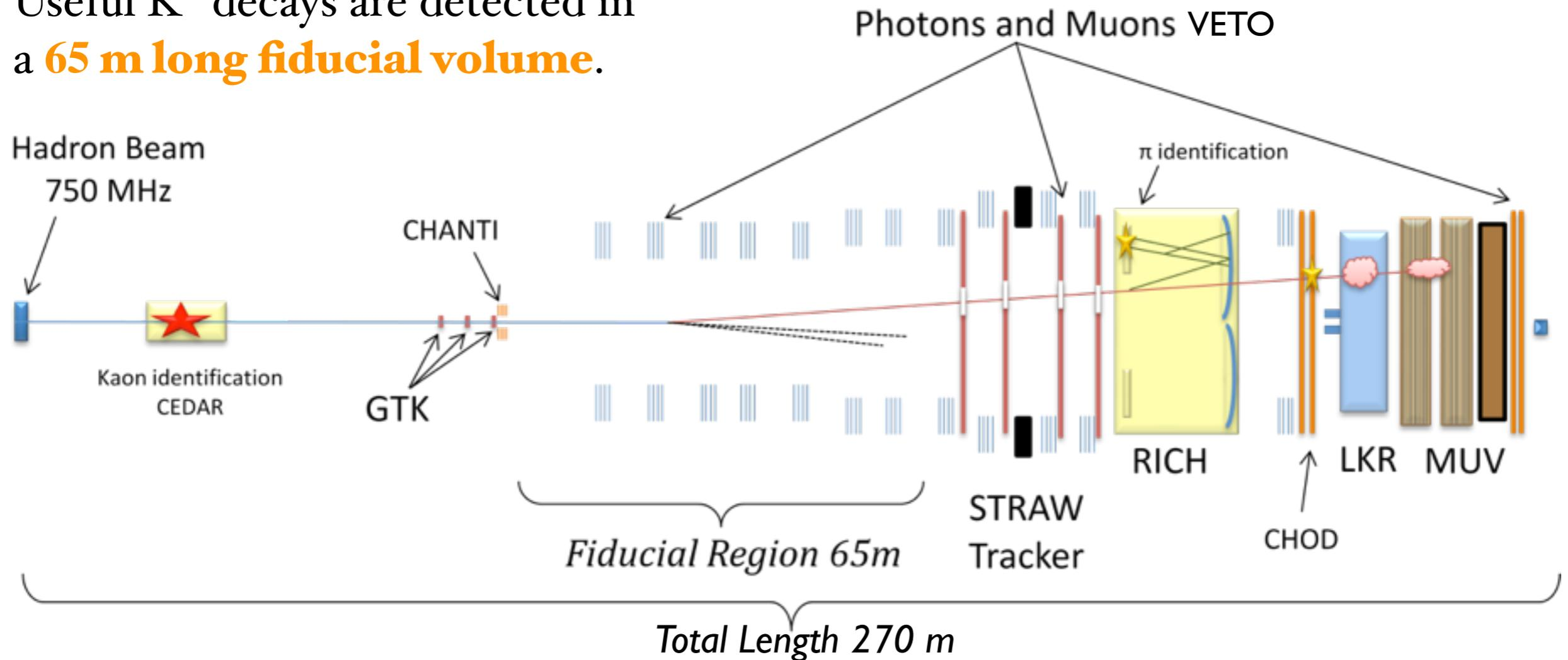
Approximately cylindrical shape around the beam axis for the main detectors. Diameter varies from 12 to 220 cm, in order to let the very intense flux of **undecayed beam particles passing through**.
