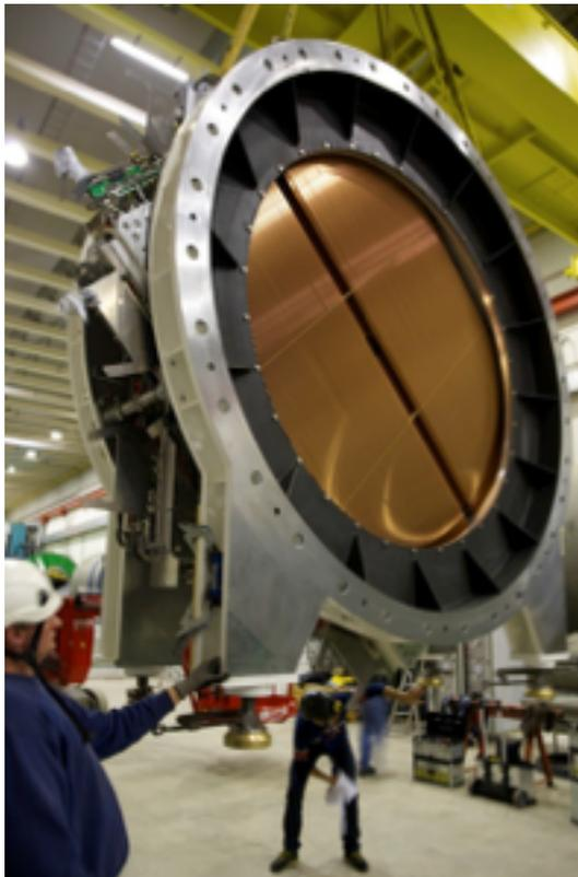
4 chambers in vacuum, 7168 STRAW tubes with  $\varnothing 1\text{cm}$ , 4 layers per chamber ( $< 0.5 X_0$ ). Magnet after the 2<sup>nd</sup> STRAW chamber provides a 270 MeV/c momentum kick in the horizontal plane.
