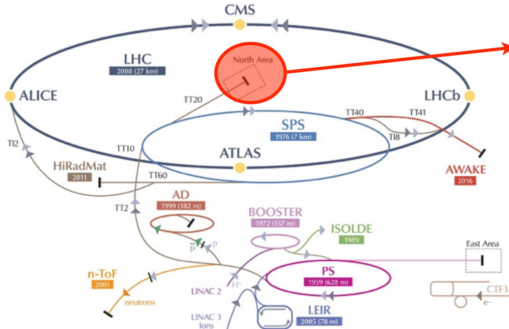
The NA62 is housed in the CERN North Area. A new beam line provides a secondary charged hadron beam 50 times more intense than in the past, with only 30% more SPS protons on target
