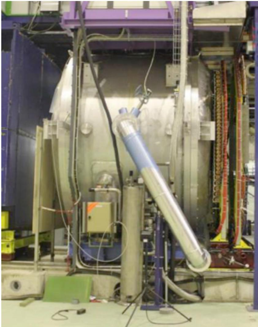
*Ionization chamber + liquid Krypton, 2x2 cm<sup>2</sup> cells. Inherited from NA48 and equipped with new readout electronics.*
