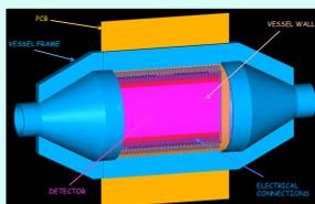
2. vessel with thin cylindrical kapton walls (<100 μm) where nitrogen is circulated  $\rightarrow$  quite uniform temperature distribution across sensor area
