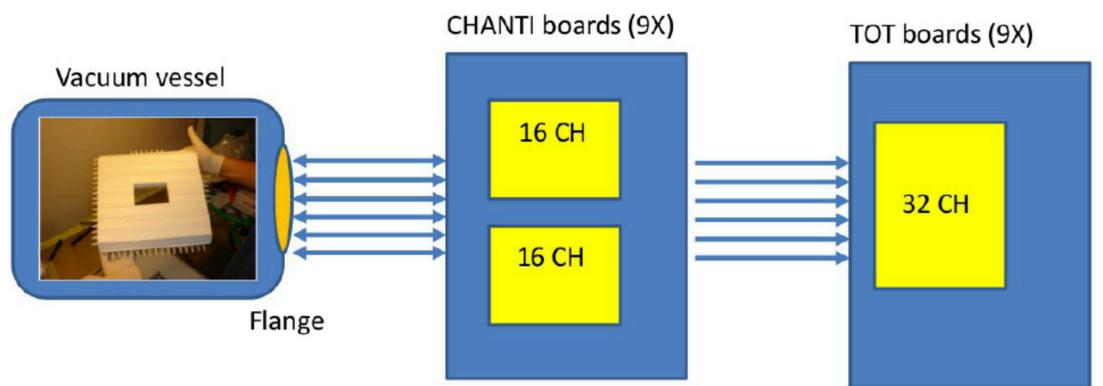
Preliminary tests have been done with cosmic rays using the first prototype station and a the FEE prototype board. External trigger has been used. About 120 photoelectrons have been collected for each layer. Time measurements, corrected for time slewing using TOT measurement, have shown a resolution of the order of 800 ps.
