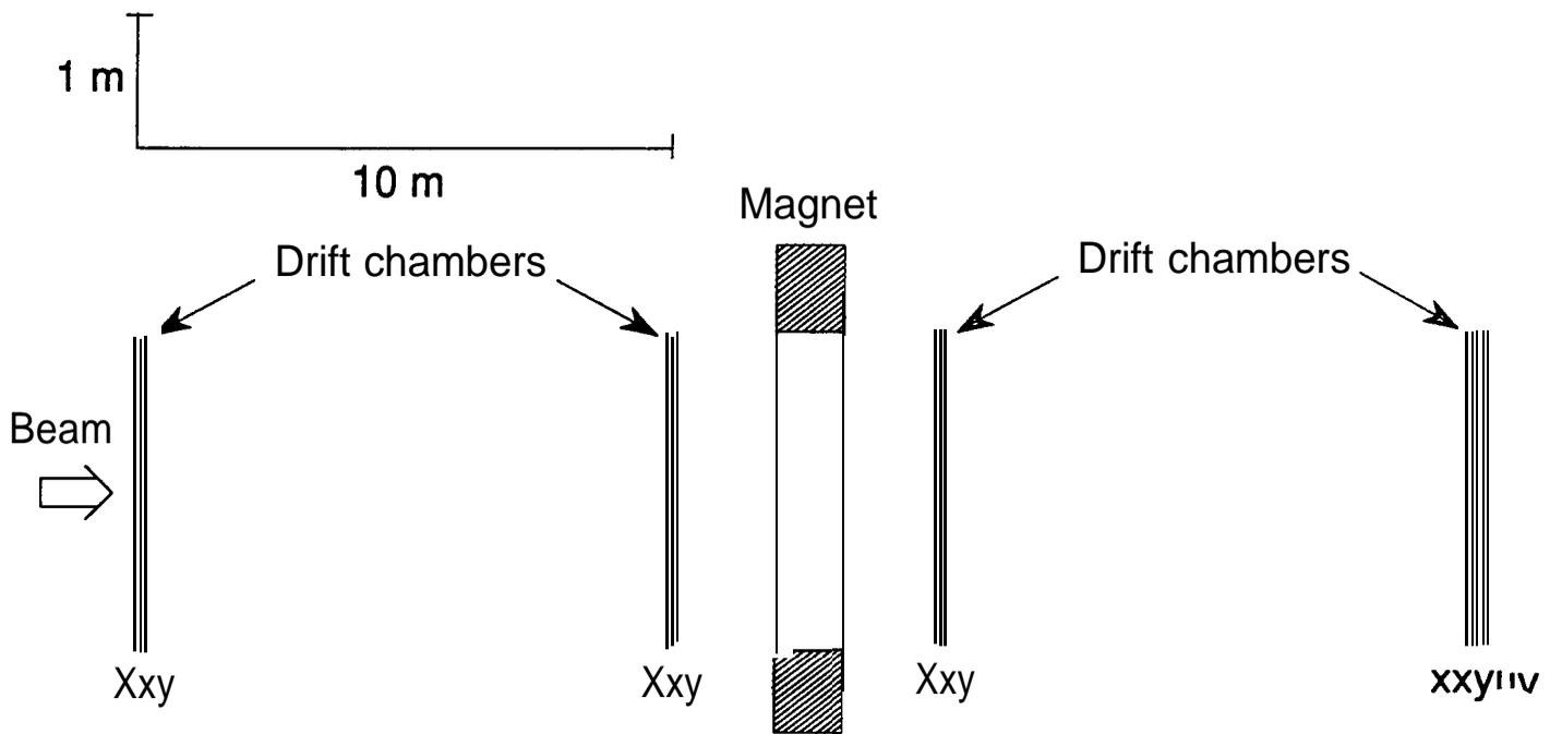
**Fig. 8** Disposition of chambers and wire planes in the magnetic spectrometer
