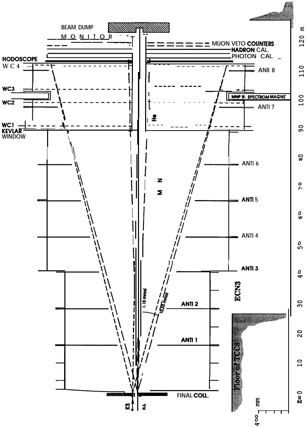
Fig. 2 Schematic layout of vacuum tank and spectrometer with arrangement of anticounter "pockets" (vertical section)
