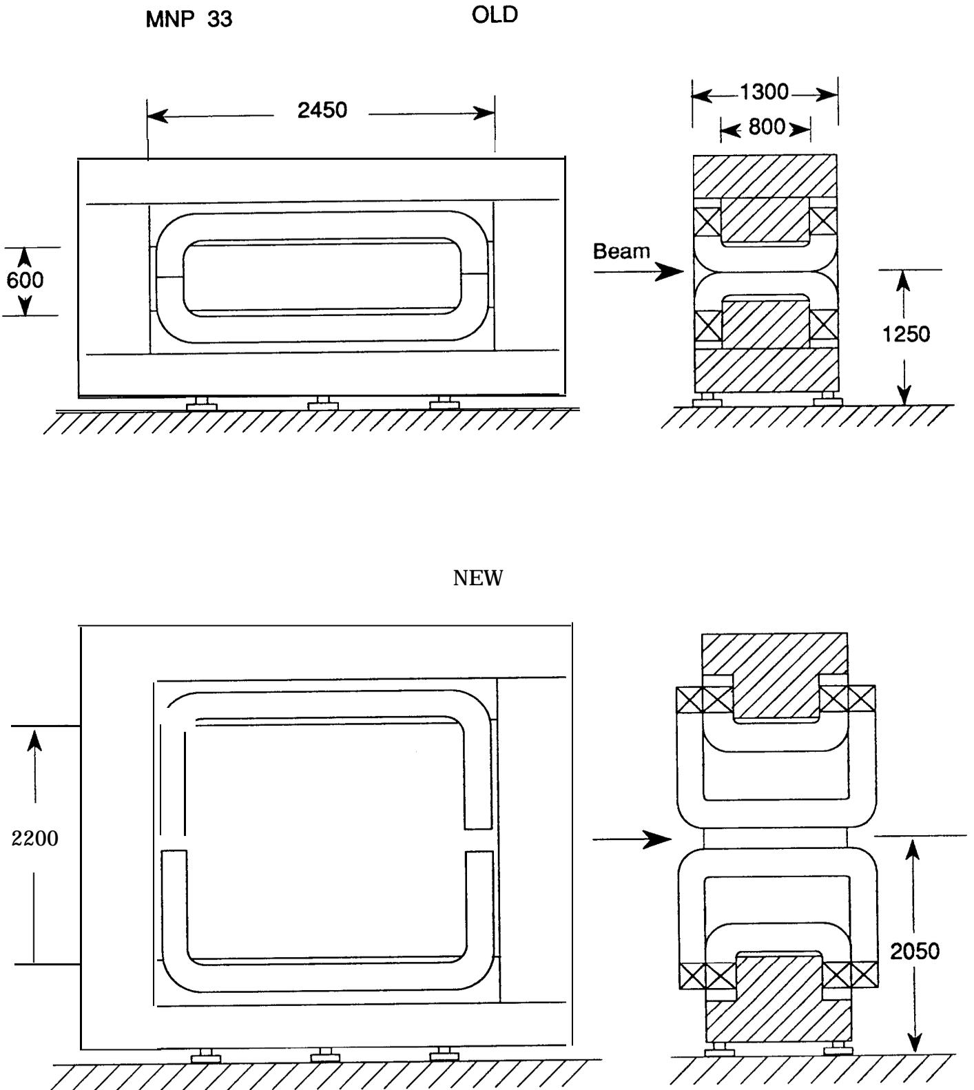
Fig. 9 Spectrometer magnet with increased gap and additional coil in the original (top) and the modified version (bottom)
