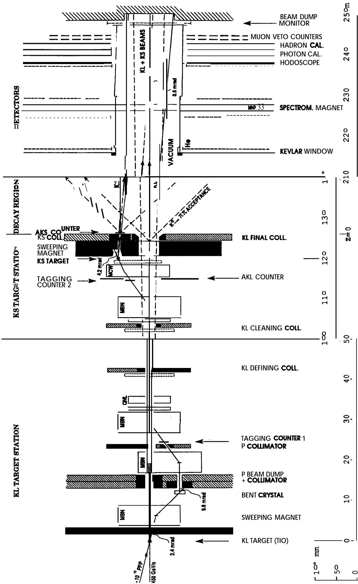
Fig. 1 Schematic layout of combined  $K_L$  and  $K_S$  beams (vertical section)
