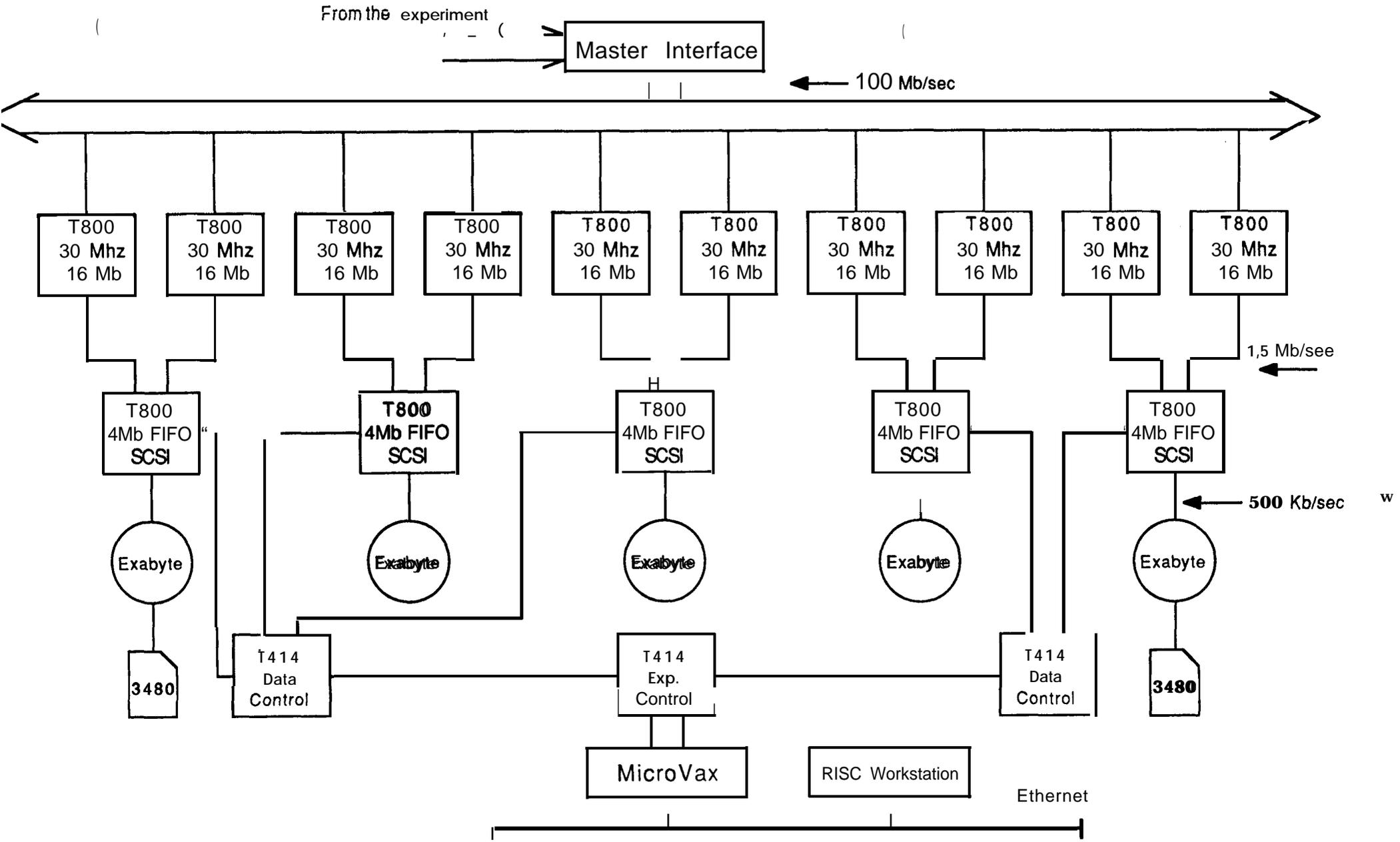
Fig. 13 Data acquisition read-out scheme
