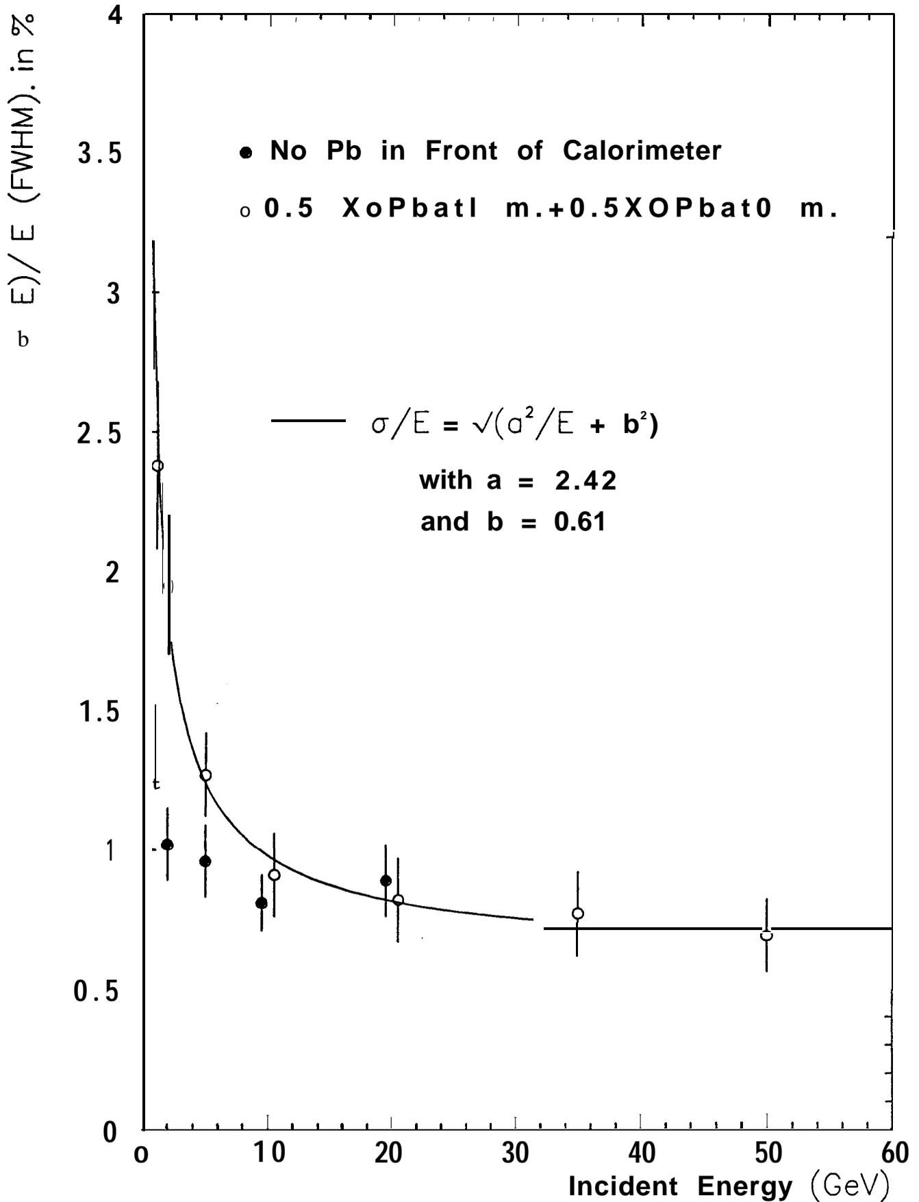
Fig. 6 Resolution of liquid xenon calorimeter
