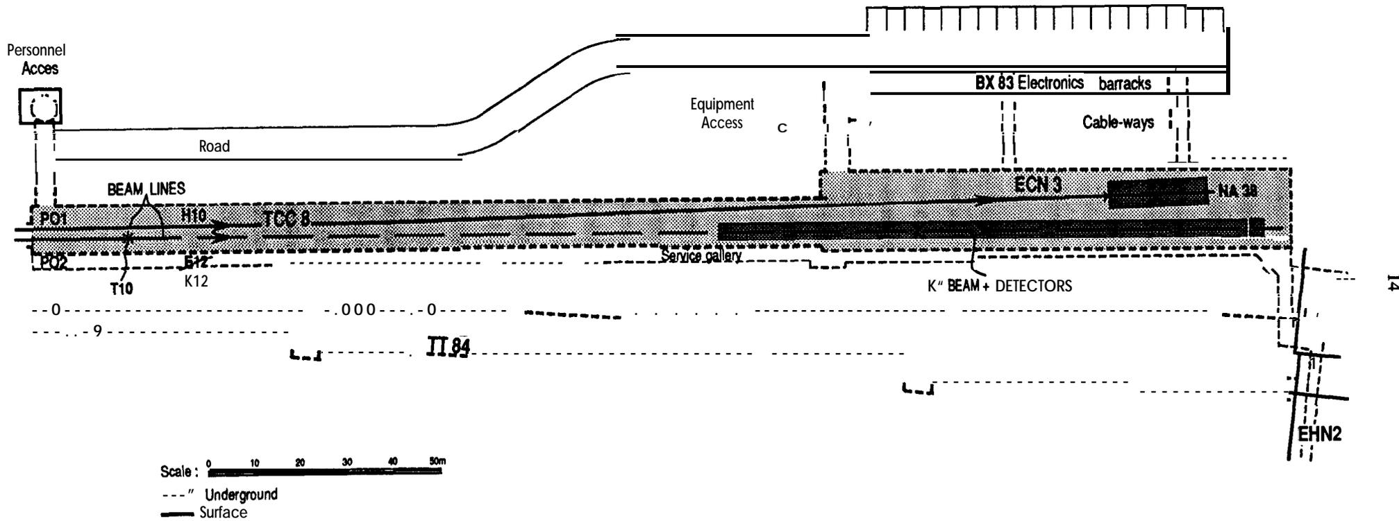
Fig. 5 Proposed layout of  $K^0$  beam in North Area High Intensity Facility
