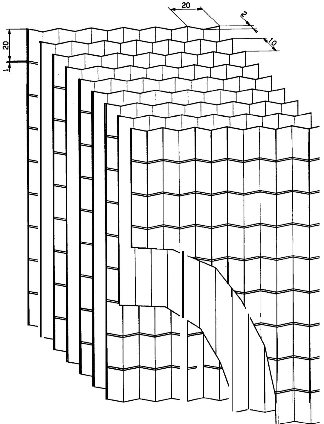
Fig. 7 Electrode structure of the liquid xenon calorimeter for particles entering from the left
