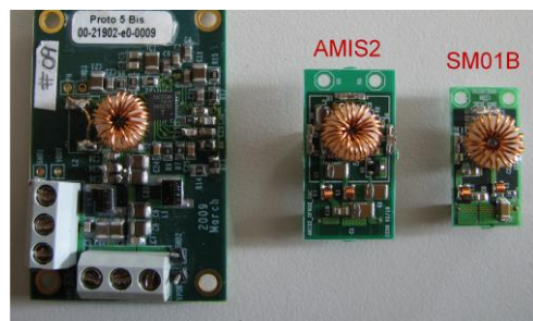
Figure 20: DCDC converter prototypes developed at CERN, Proto5 (left), AMIS2 EMC (center) and SM01B (right).
