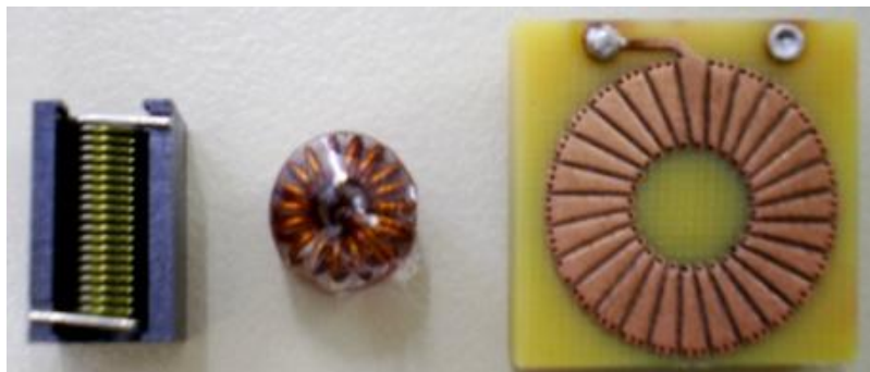
Figure 24: Solenoid, hand wrapped and PCB toroid inductors.
