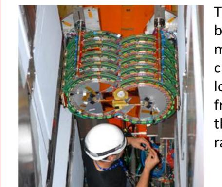
The T2 telescope is based on gas electron (GEM) multiplier chambers and located at ±13.5 m from IP5 and covers the pseudorapidity range  $5.3 \le \eta \le 6.5$ .
