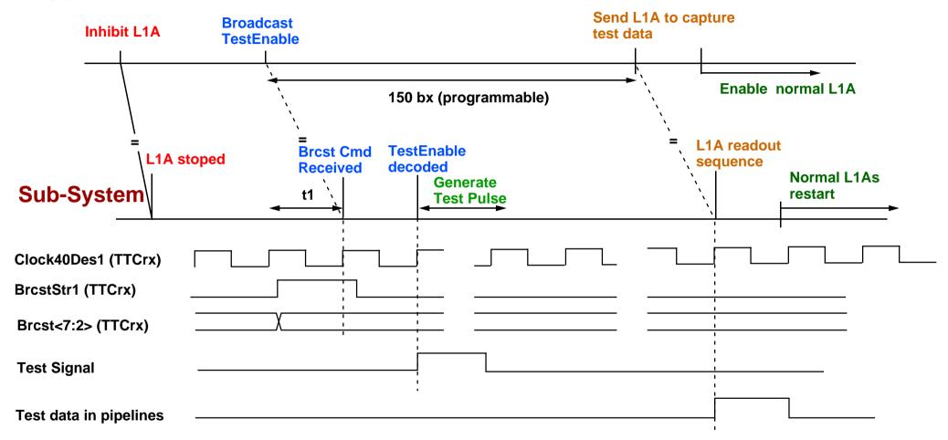
t1 = delay on TestEnable command; adjusted in subdetector TTCvi's
