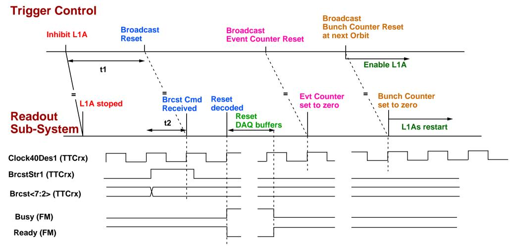
t1 = time needed to empty DAQ buffers in subsystems
