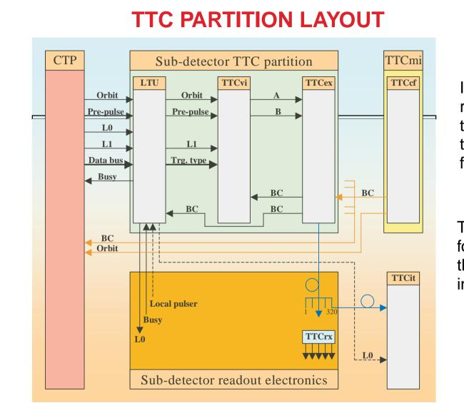
In order to write rapidly to the TTCvi, the LTU must be able to be a VME master for such transmissions.
