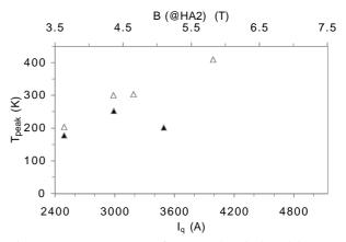
Figure 4:  $T_{peak}$  vs.  $I_q$  for quenches induced by HA2. Quenches at 4.3 (1.9) K are shown as filled (open) symbols.
