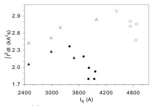
Figure 5:  $\int I^2 dt$  vs. I<sub>q</sub> for spontaneous (circles) and heater HA2 induced (triangles) quenches. Quenches at 4.3 (1.9) K are shown as filled (open) symbols.
