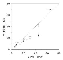
Figure 3:  $v_q$  measured by initial dR/dt vs that by  $\Delta t$  for heater HA2 induced (triangles) and natural(circles) quenches. Quenches at 4.3 (1.9) K are shown as filled (open) symbols. The open squares give the  $v_q$  measured by average dR/dt for the same quenches plotted directly below them.
