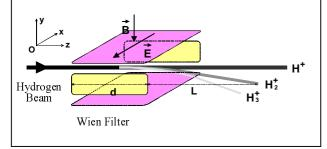
*Figure 3*: Schematic design of the Wien mass separator.
