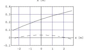
Fig. 4: Ejection (solid line) and central trajectories (dotted line) through the field map.
