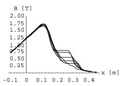
Fig. 2: Calculated fields for the five shimmed and un-shimmed blocks over the range -0.1 m  $\leq$  x  $\leq$  0.5 m.
