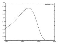
Figure 1: Radiation spectra from an electron shortly after the entrance in a positron bunch.
