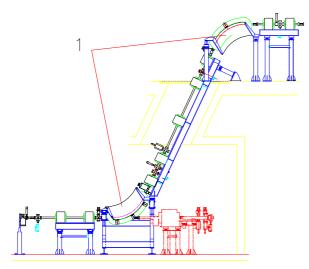
Fig. 2 Transition of under ground level and ring level, with 65° dipole (1) for deflection
