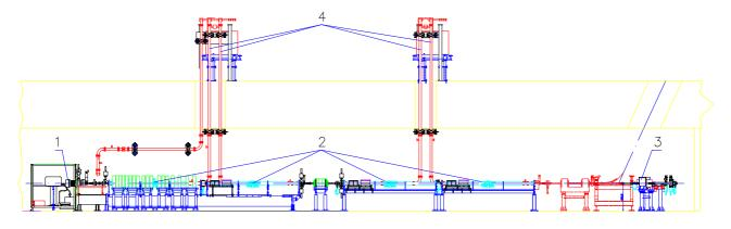
Fig. 1. Linac: CAD drawing of the gun (1), the linear accelerator strutures (2), the spectrometer (3) and the wave guide of RF system (4)
