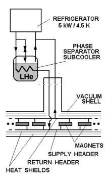
Figure 3: A possible unit of  $2 \times 5$  km long of cryomagnetic system for a multi-TeV range accelerator
