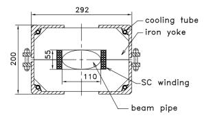
Figure 2: Cross-section of the Nuclotron dipole
