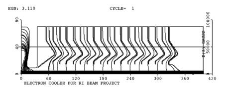
Figure 1: Electron gun with magnetic field 5T and acceleration voltage 300kV (unit: mm in length)
