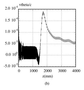
Figure 3: Transverse electron velocity starting 5.5mm off axis. (a) is radial and (b) is azimuthal velocity.
