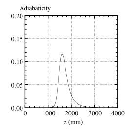
Figure 4: Adiabaticit parameter in this electron cooler
