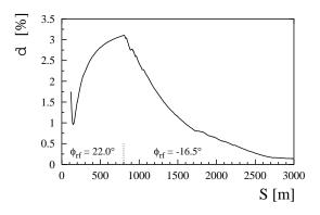
Figure 1: Typical BNS relative energy spread  $\delta$  along the SLC linac.
