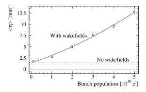
Figure 2: Expected dispersion  $\langle \eta \rangle$  in the end of the SLC linac as simulated for different SLC bunch currents. The wakefield-free dispersion is indicated by the dotted line. The SLC linac dispersion is driven by wakefields.
