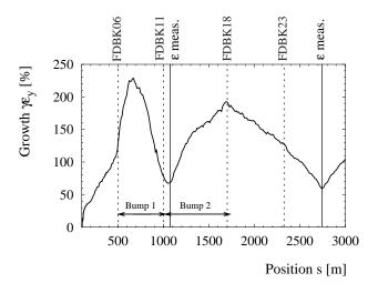
Figure 3: Overview of emittance measurement and optimization before the 1997/98 run. The beam emittances were minimized mainly on the wires in the middle and after about 90% of the linac length, using bumps mainly in the first half of the linac. The vertical beam emittance almost doubles in the uncorrected region of the linac.
