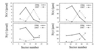
Figure 4: RMS variation S of the different feedback setpoints x', y' (left) and x, y (right) over three month periods in 1996 and 1997. The feedback position and angle offset introduce trajectory oscillations (= emittance bumps) up to the next feedback. The electron and positron setpoint variations are averaged. The bias towards later bumps is clearly seen for the new 1997/98 tuning approach.
