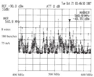
Figure 8: Measured mode spectrum from 400 to 600 MHz, rf-shielding: 8 wires, resolution bandwidth 100 kHz.
