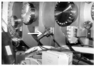
Figure 4: Loop antenna at one of the flanges of the vertex chamber.
