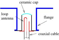
Figure 5: Schematic view of the loop antenna.
