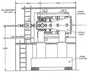
Figure 1: The HERA-B Vertex Chamber.
