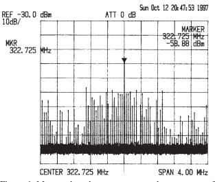
Figure 6: Measured mode spectrum around a resonance of 322.75 MHz. Rf-shielding: 4 strips, resolution bandwidth 1 kHz.
