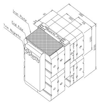
Figure 2: Th geometrical configuration of magnet structure and end pole.
