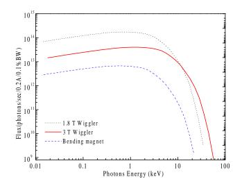
Figure 1: Comparison of photon energy and flux between the wiggler and the bending magnet.
