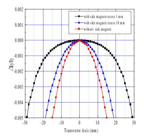
Figure 3: The field uniformity along the transverse axis with side magnets.
