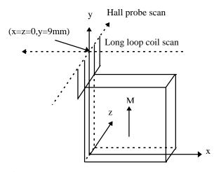
Figure 2: V-type block measurement procedure by the Hall probe and the translation long loop coil method.
