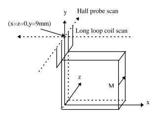
Figure 1: H-type block measurement procedure by the Hall probe and the translation long loop coil method.
