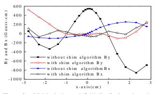
Figure 3: Multipole integral field distribution along the transverse x-axis with and without shim algorithm.
