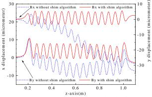
Figure 4: Electron trajectory along longitudinal z-axis with and without shim algorithm.
