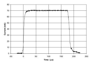
Figure 3. Hydrogen-ion beam pulse. The beam pulse was generated by pulsing the hydrogen discharge with a current-regulated voltage pulse to the magnetron cathode.
