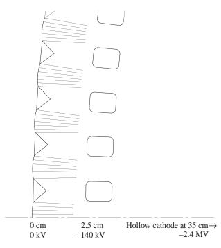
Fig. 3. Model for concentric annular preaccelerator grids.
