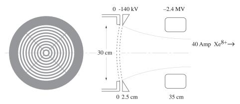
Fig. 2. High perveance extractor concept for laser ion source with magnetic bucket, showing concentric annular grids.
