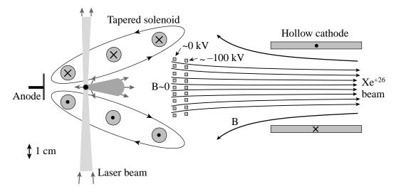
Fig. 1. A conceptual method of extracting highly-charged ions created by a short-pulse laser. Frozen Xenon targets  $\sim 10 \ \mu m$  in radius are prepulsed by a low energy laser and expanded well below the critical density before the main pulse. Typical numbers for the main laser: 0.5  $\mu m$ , 100 fs, 1 petawatt. The tapered solenoid field directs ion flow toward the concentric annular extractor grids, which are adjusted radially to control beam aberrations.
