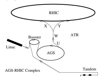
Figure 1: Schematic layout of the AGS-RHIC complex.
