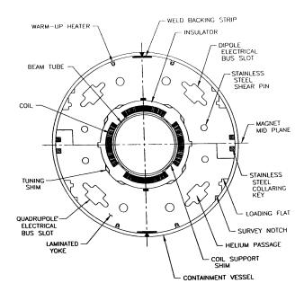
Figure 6: Triplet quadrupole cross-section showing empty slots for tuning shims.
