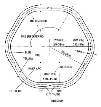
Figure 2: Layout of the RHIC collider and the tunnel.
