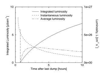
Figure 9: Integrated, instantaneous, and average luminosities during a nominal store of gold ions.
