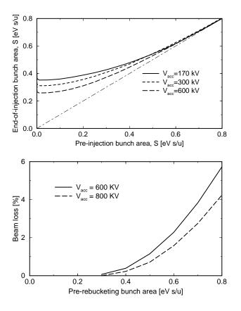
Figure 8: (Top) Growth in longitudinal area of a gold beam due to intra-beam scattering during the two minute injection period. (Bottom) Beam loss during re-bucketing as a function of initial bunch area, for nominal (600 kV) and potential (800 kV) excitations of the 28 MHz RF system.
