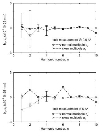
Figure 4: Arc dipole magnetic field multipole harmonics at injection (0.6 kA) and storage (5 kA) currents. Harmonic n = 1 is quadrupole.
