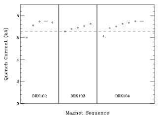
Figure 7: Training curves for the first three DX beam splitting magnets.
