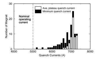
Figure 3: Arc dipole quench current distribution.
