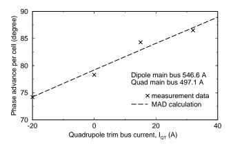
Figure 5: Measured and predicted phase advance per cell.
