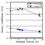
Fig. 3: Steerer calibration versus sextupole current.
