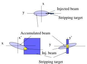
Fig.1. Transverse phase space filling at the beam multiturn injection into U-10 ring.
