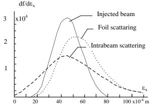
Fig.2. Horizontal emittance growth under beam scattering in foil and IBS ( $A_{z}=1.1 \ 10^{4} \text{ m rad}$ ).
