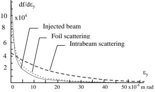
Fig.3. Vertical emittance growth under beam scattering in foil and IBS ( $A_y=60 \ 10^{-4} \text{ m rad}$ ).
