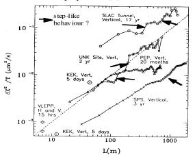
Figure 4 : Differential movement as a function of distance in a number of machines for several observation periods.
