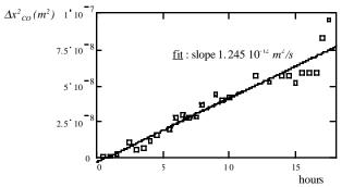
Figure 5 : Orbit deformation  $\Delta x_{co}^2$  versus time in LEP, where fit is compatible with  $L_{ch}=1.6 L_{cell}=130 m$ .
