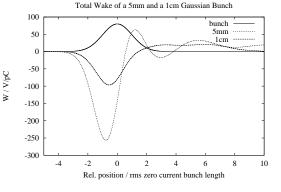
Figure 2: The wake field (all components) of a 5 mm and a 1 cm Gaussian Bunch.
