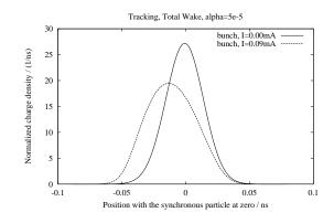
Figure 3: The average normalised charge density over the last 500 turns as seen by a tracking run with  $N_{\rm par} = 100\,000$ . Total wake for  $\alpha = 5 \times 10^{-5}$ , design current.
