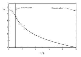
Figure 1: Repulsive potential of the uniformly charged beam in a round chamber.
