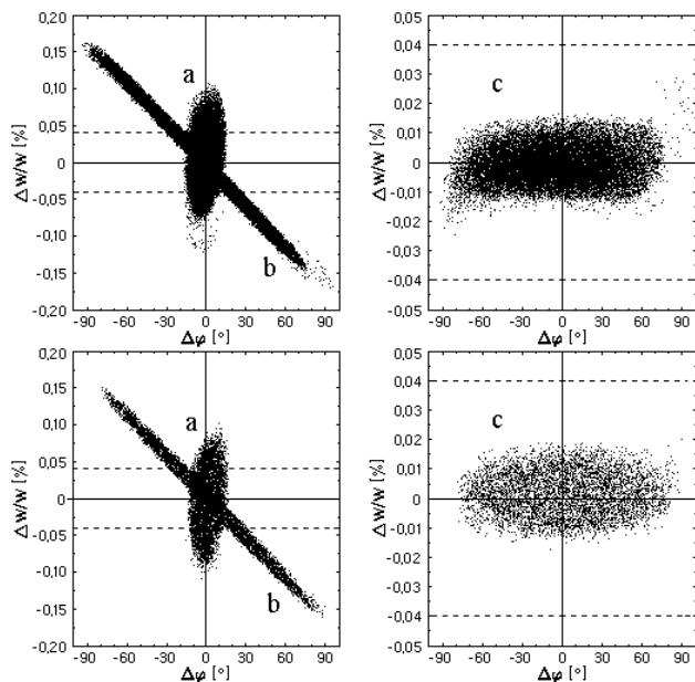
Fig. 6: Longitudinal phase space: a) at linac end; b) at transfer line end; c) after linear rotation. Up: for 20,000 particles with 6d waterbag input and errors. Down: for 5000 particles with 4d-2d waterbag input and no errors.
