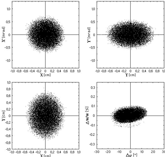
Fig. 4: Output distribution at the linac end for 20,000 particles; 6d waterbag input, phase and amplitude errors.
