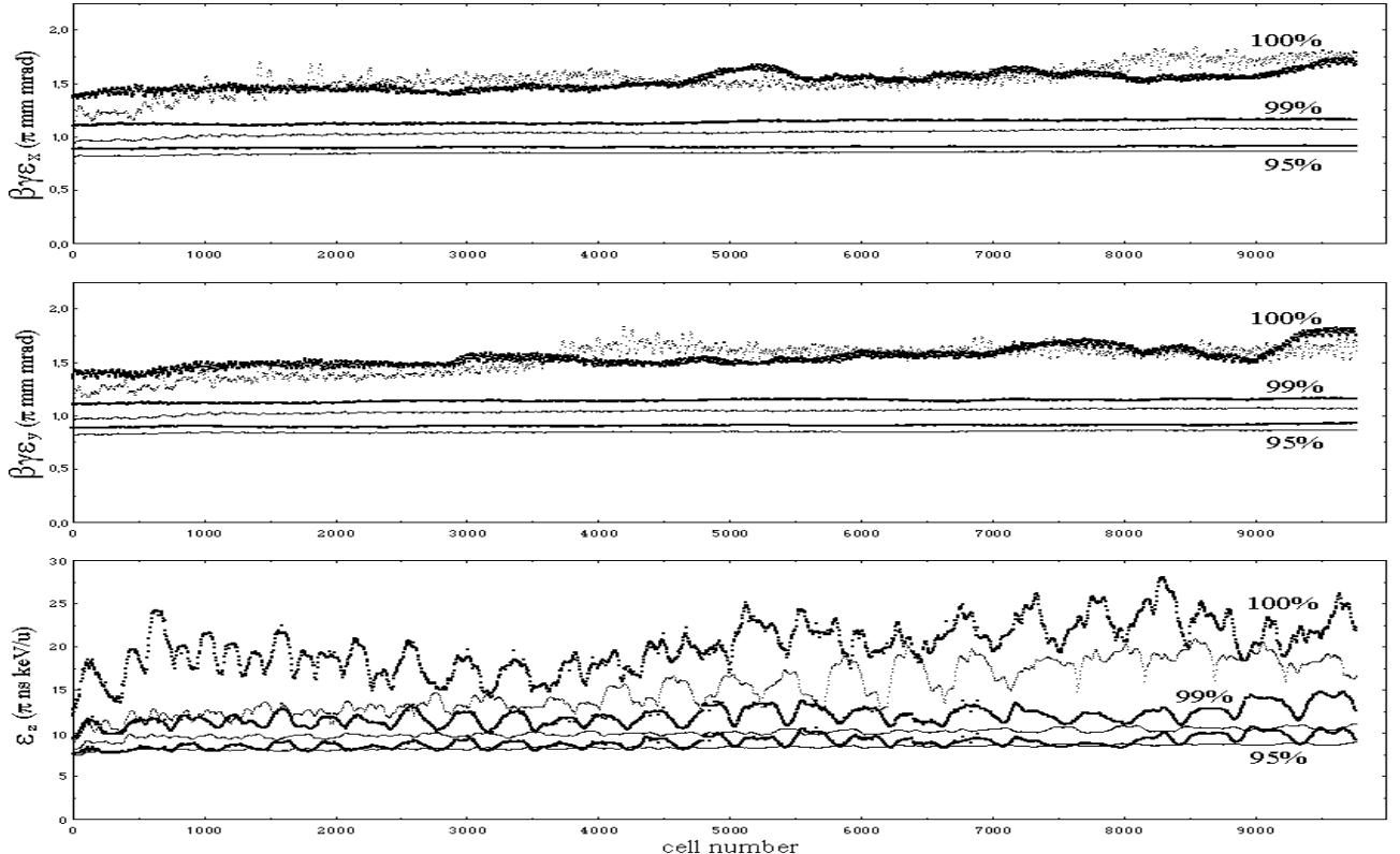
Fig. 3: Full (100%, 99%, 95%) emittance along the linac for a 6d waterbag input with 20,000 particles, including errors (bold curves) compared to a 4d-2d waterbag input with 20,000 particles and no errors (light curves).
