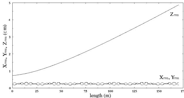
Fig. 5: Bunch rms length and radius along transfer line.
