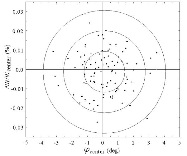
Fig. 2: Center of bunch position with uncorrelated amplitude and phase errors: *Left:* along the linac with 20,000 particles and full current. *Right:* at linac output with 5000 particles and no current (statistics over 100 different sets).
