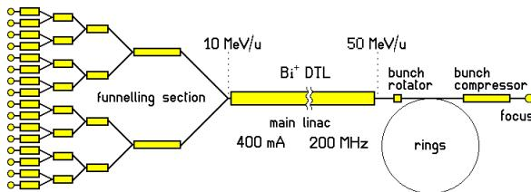
Fig. 1: Scheme of the heavy ion driven inertial fusion.
