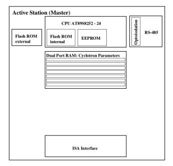
Figure 2: CtrlBUS controller block diagram.
