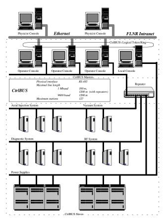
Figure 1: The integration of CtrlBUS in a control system of FLNR
