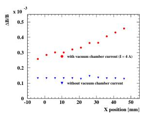
Figure 3: The magnetic field profiles in the horizontal plane transverse to the beam (x direction). Dots: Field perturbation due to train current. Triangle: Remaining field after the train current excitation.
