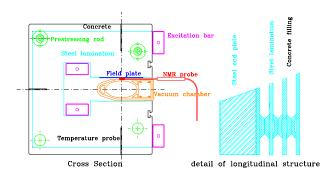
Figure 1: Cross section of the instrumented LEP dipole. The iron-concrete structure is shown on the right side.
