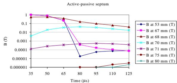
**Figure 6.** Evolution with time of the stray fields at different points of the active-passive septum magnet model for the LLS, calculated with OPERA-2d<sup>®</sup> tr.
