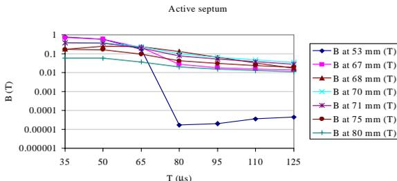
**Figure 4.** Evolution with time of the stray fields at different points of the active septum magnet model for the LLS, calculated with OPERA-2d<sup>®</sup> tr. The position with
