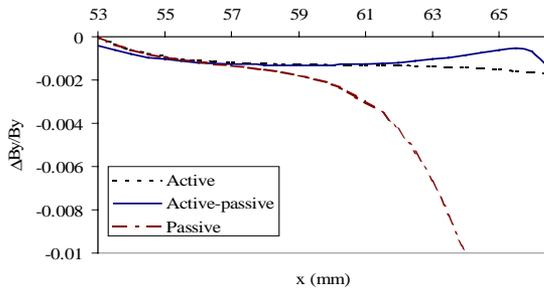
**Figure 3.** Relative variation of the vertical field in the aperture of the two LLS septum models: the passive and the active-passive. Note that the path of the electrons occurs in this region of the magnet aperture.
