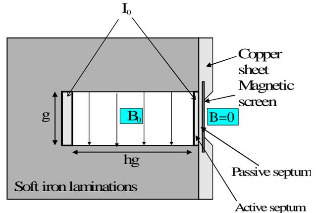
**Figure 1.** Cross-section of an active-passive septum magnet. The current in the coils,  $I$ , is pulsed. The stray fields are screened in the copper sheet by eddy currents and by the ferromagnetic screen. The cooling system is not shown.
