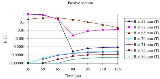
**Figure 5.** Evolution with time of the stray fields at different points of the passive septum magnet model for the LLS, calculated with OPERA-2d<sup>®</sup> tr.
