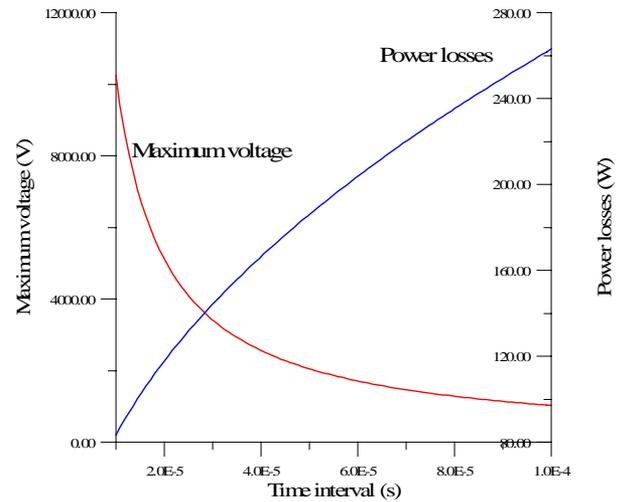
**Figure 2.** Maximum voltage and power losses as a function of the pulse duration  $\tau$  for the active-passive septum magnet proposed for the LLS.
