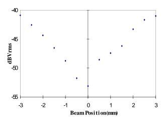
Figure 1: Beam position signal (dBVrms) versus beam position (mm).
