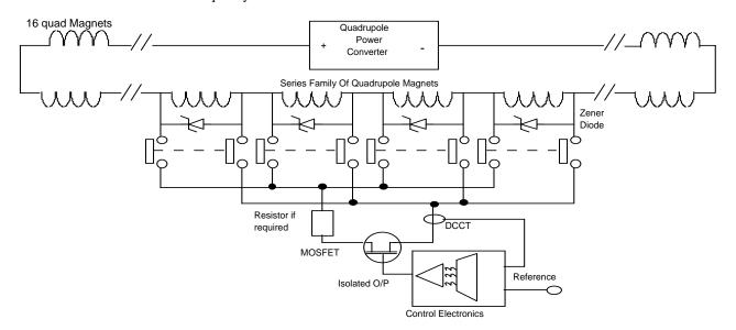
Figure 3: a.c shunt design with common power and control electronics for four quadrupole magnets
