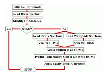
Figure 3. Execution Flow Diagram.
