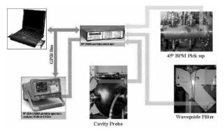
Figure 1. Measurement System.
