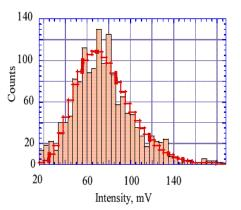
Fig. 3. Measured FEL intensity distribution, together with a plot of a Gamma function distribution with M=9.
