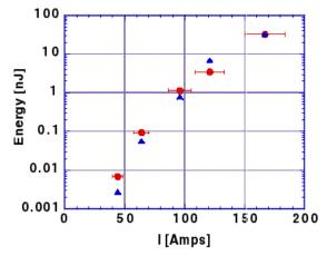
Fig. 2 Plot of measured FEL average intensity, circles, and Ginger simulations, triangles.
