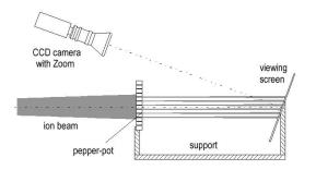
Figure 2: Schematic sketch of the pepper-pot emittance device.
