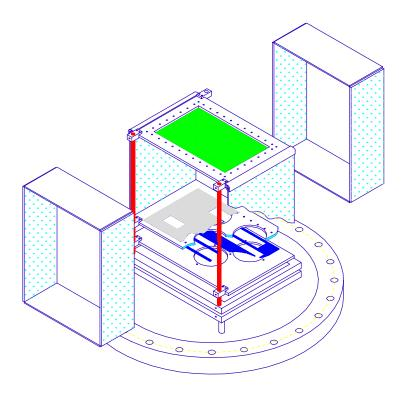
Figure 1: Schematic drawing of the SIS residual-gas beam profile monitor. Two of these monitors are used, one for horizontal and one for vertical measurements. One sees the plates for the back-bending fields in front the detector as well as behind the detector. For simpler assembly, the complete detector is mounted on a flange. The Germanium coated glass plates at the edge of the detector as well as at the edges of the compensation plates serve as voltage dividers.
