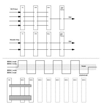
Figure 2: Schematic drawing of the analog electronic and the data acquisition system.
