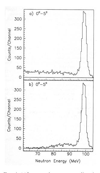
Figure 4: (a) Reconstructed energy spectrum of incoming neutrons, using a proton spectrum in the angular range  $0-5^\circ$ , obtained with a CH<sub>2</sub> target, and subtracting the contribution from the  ${}^{12}C(n,p) {}^{12}B$  reaction. (b) The same spectrum as in (a) using TOF-gating.
