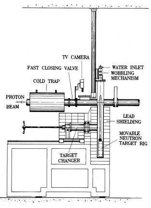
Figure 2: Neutron-source arrangement
