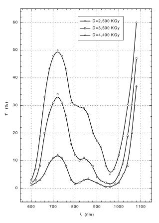
Figure 3. The transmission spectral data of a LiF monocrystal, irradiated by electrons at various irradiation doses.
