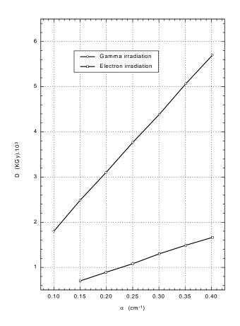
Figure 1. The variation of the absorption coefficient for  $\text{LiF:}F_2^-$  crystals at 1.064µm wavelength, function of the irradiation dose, with gamma and electron radiation.
