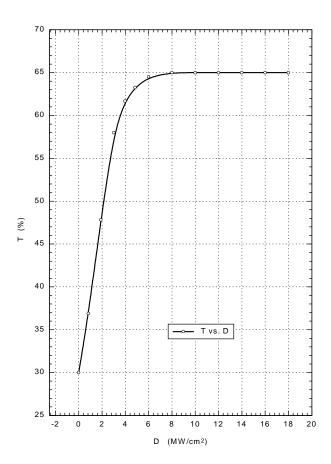
Fig. 2. The non-linear variation of transmission in a  $\text{LiF:}F_2^-$  crystal function of the incident laser pulse power density.
