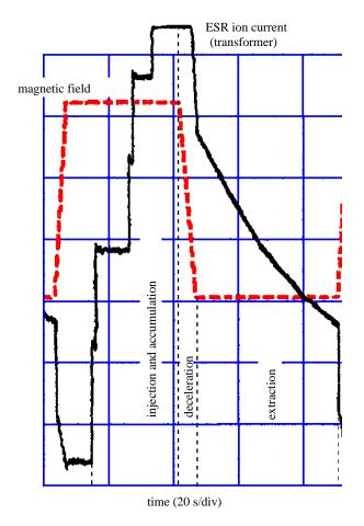
Figure 4: Typical ESR cycle for experiments with decelerated beams and charge exchange extraction.
