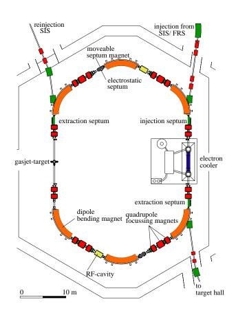
Figure 1: Storage ring ESR with its main components.
