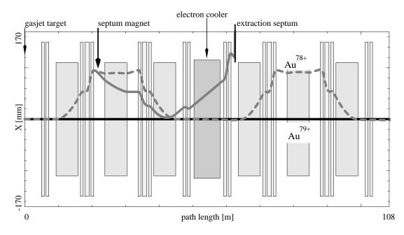
Figure 2: Horizontal separation of the orbits of a primary and secondary Gold-beam along one revolution in the storage ring. The extracted secondary beam is deflected into the extraction septum by a small kick in the north bend of the ESR.
