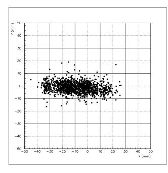
Figure 1: Spatial distribution of the photons at the photon detector
