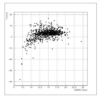
Figure 2: Dependence of electron vertical displacement at electron tagger plane on electron energy
