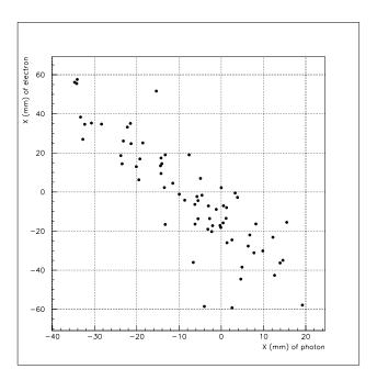
Figure 3: Scatter plot of the horizontal displacement of the bremsstrahlung photons at PD vs the horizontal displacement of the secondary electrons at ET
