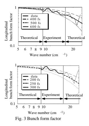
The dashed curves in Fig. 3 represent those of three bunch length (400, 500 and 600 fs at FWHM). We used the measured bunch form factor in the range of 9.5 - 18 cm<sup>-1</sup> and the theoretical bunch form factor out of the range for the analysis. In this case, we adopted the
