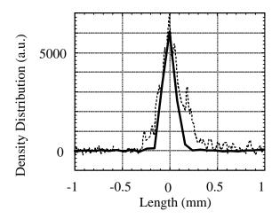
Fig. 4 Bunch distribution by the interferometry (solid) and that by the streak camera (dashed)
