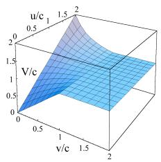
Figure 3: Three-dimensional plot of the composed velocity V (axis z), following the present work.
